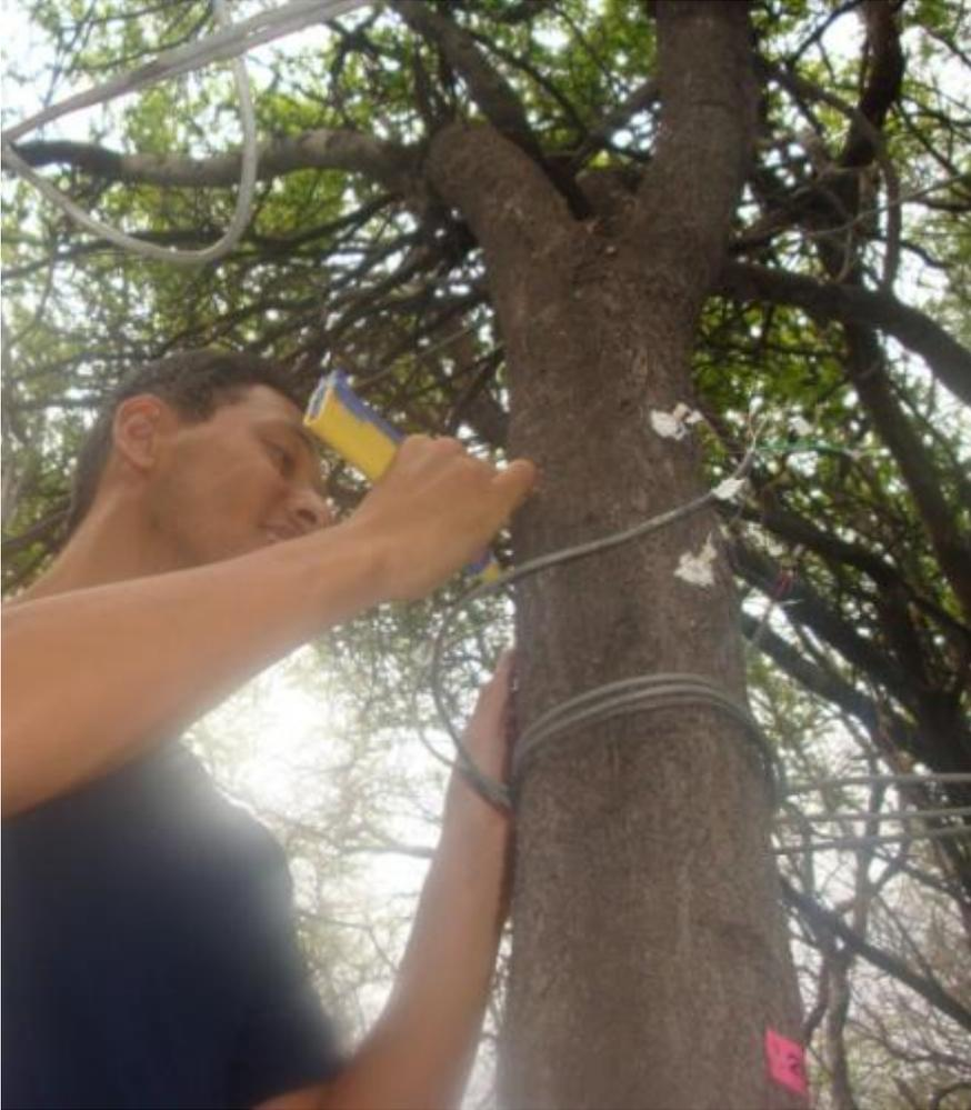
Dr. Yoshiyuki Miyazawa installing sap flux probe at a previous site; protocol from previous work informed the sampling design for this project.
