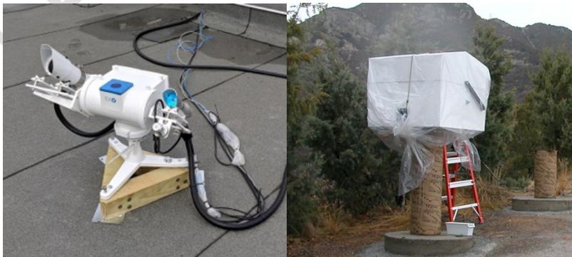
Figure 4: Left: the integrating sphere and sun-tracking mount. Right: example enclosure design based on commercial product at another site.
