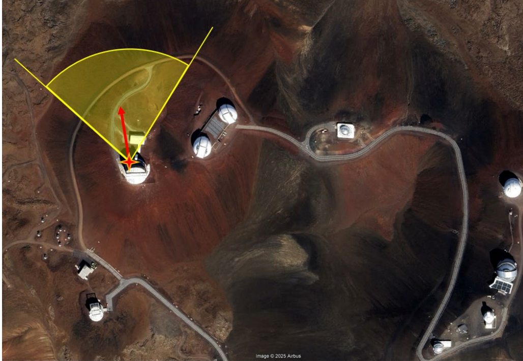
Figure 5. Visibility plot of the illuminator. It is effectively blocked by the elevator tower and the door structure on the dome. The illumination angle is roughly 90 degrees.
