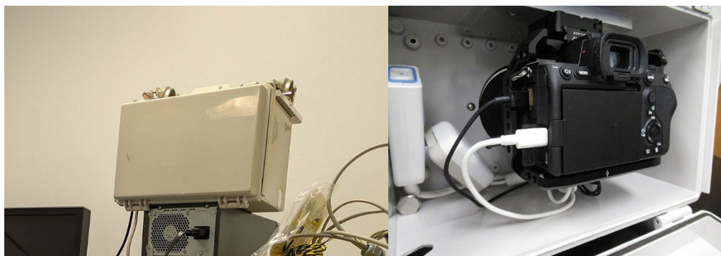
Figure 6: Subaru "Cloudcam" under testing. The size is 30cm x 22cm x 15cm.
