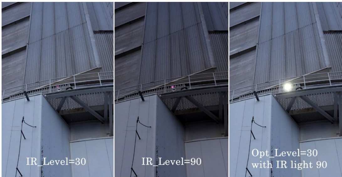
Figure 4. the view of the test illumination. The right and middle panels show the visibility of the IR light with the IR_Level=30 (medium) and 90 (maximum). For the actual use, the IR_level less than 10 is enough for the fog detection (based on our on-site test during 2020-2021). For comparison, we show the view of the regular white light that has similar brightness to the small pen light. It demonstrates the effectiveness of the IR light for no-impact operation.
