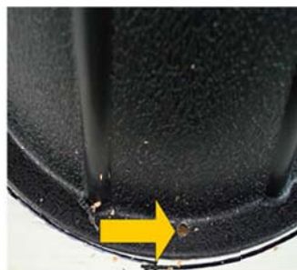
When screwing in the lifts, it is best to drill a hole through the lift. (The board needs a smaller drill bit, it is best to just screw into board without pilot hole.)
