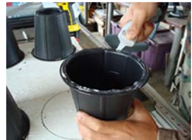
A bead of sealant should be applied at the base of lifts before screwing in to keep rain water from filling the lifts.
